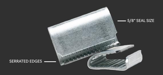
Our open galvanized metal seals for polyester or PET strapping have a serrated design on the inside of the seals so that it grips into the strap when crimped with the sealer. Our serrated seals are designed to be used with a sealer or crimper, forming a heavy duty grip on polyester strapping. Only compatible with a 5/8" deluxe strapping sealer.
